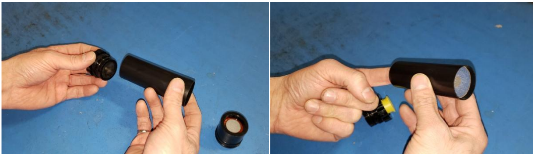
Figure 3: Optional removal of nozzle to extract propellant grain.
