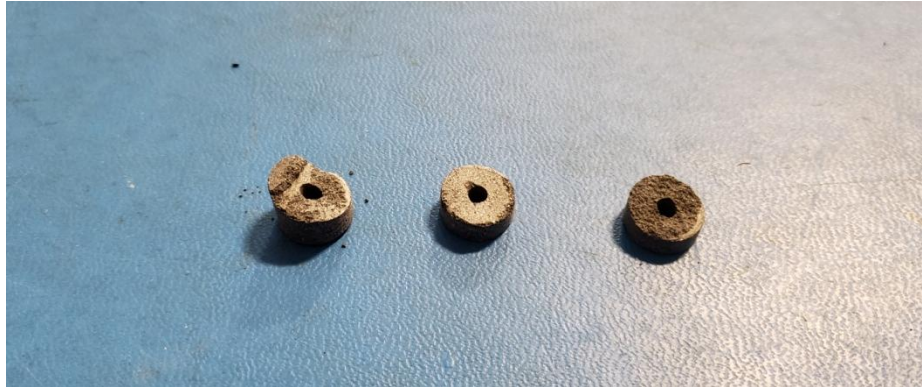
Figure 11: Pellet examples after cutting (LEFT) not cut perfectly and oversized (CENTER) additional trimmed pellet (RIGHT) as cut pellet approx 50%.
