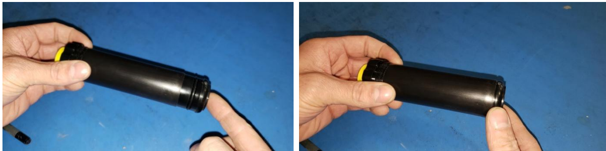
Figure 14: Re-assembly of propellant grain (LEFT) correct forward facing orientation (RIGHT) wrong orientation
