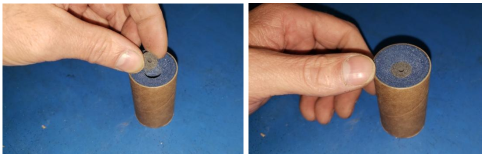
Figure 12: Pellet cutting procedure, scoring the OD by rolling the pellet with light pressure
