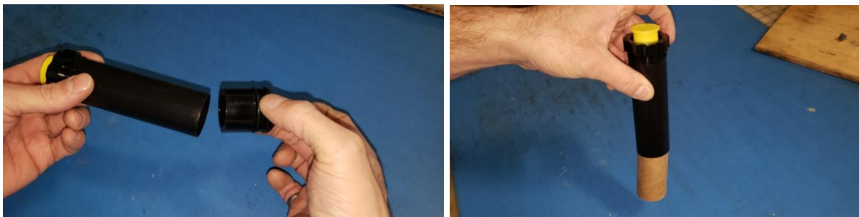
Figure 2: (LEFT) Forward closure removal (RIGHT) sliding grain out from liner in vertical position.
