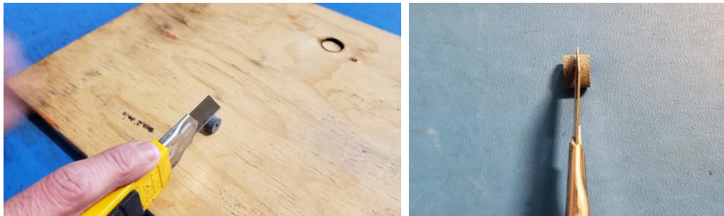
Figure 8: Pellet cutting procedure.
